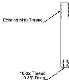
4. Install a 10-32 x 1/2" set screw into the threaded hole in the end of the stud.
