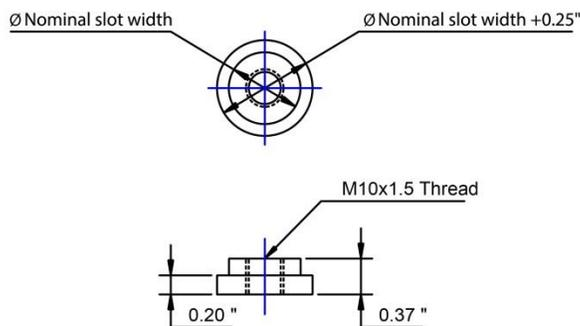
We can't tell you the dimensions, except that the center hole must be tapped M10x1.50 thread. The tap is our P/N 4838. Measure your T-slot and make it an easy fit.
