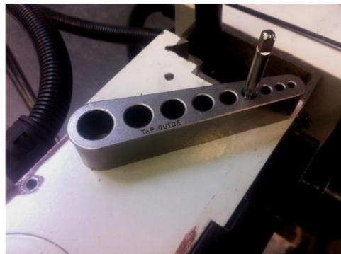
32. Clear the chips from the vertical and horizontal holes.
