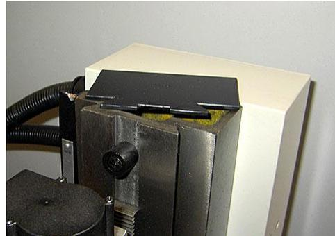
2. Drill a hole 13.38" below the top of the column casting, centered in the back of the column. Use a 9 mm, letter T, or 23/64" drill bit.
