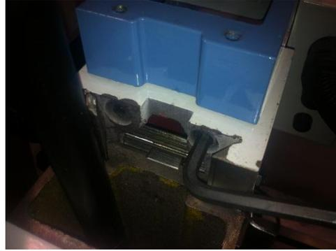
23. On the side where you removed the M8 socket head cap screw, use a 5 mm or #9 drill to drill down through the threaded hole in the belt cover and into the top of the head casting where you center punched it. You will drill into the hole for the M8 cap screw.
