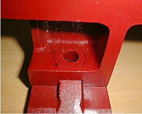
3. With the ½” transfer punch, mark the back of the casting at the center of the hole through the cam lock sleeve.
