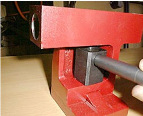
4. Remove the cam lock sleeve from the tailstock.
