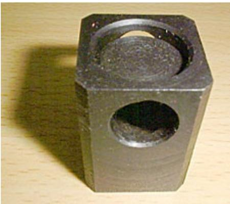
5. Put the cam lock socket and cam lock sleeve assembly on the cam lock shaft. Rotate the cam lock shaft as you slide the socket and sleeve on.
