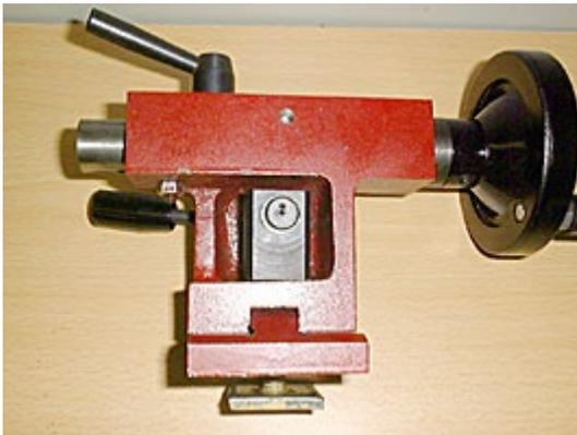
8. Put the tailstock back on the lathe and adjust the position of the clamping foot.
