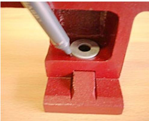
2. Using the markings made in step 1, center the cam lock sleeve sideways over the hole in the base of the tailstock.
