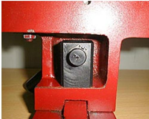
7. Screw the clamping foot into the cam lock sleeve.
