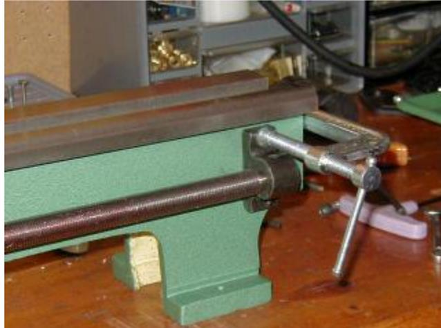
7. Move the carriage as far to the left as it will go. Engage the half nuts (handle down).
