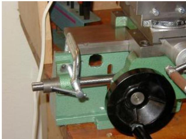
11. Engage the half nuts (handle down), and re-tighten the C-clamp to lock the right lead screw mounting bracket in the correct position.
