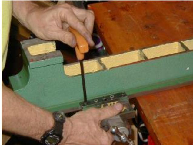
*Note: In a very few cases, the thickness of the new ways is smaller than the range of adjustment on the saddle retainer adjustment. If this occurs you will not be able to get all the play out of this adjustment. The quick fix is to place a plastic cable tie between the ways and the saddle retainer. Once things are adjusted, cinch the cable tie around the saddle retainer lengthwise. The cable tie provides a good bearing surface.*
